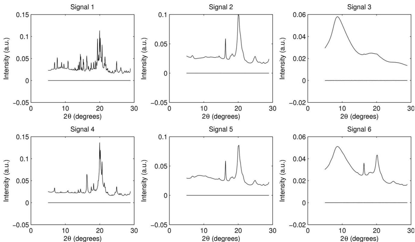
**Figure 4** Source signals extracted by applying the hierarchical scheme based on NMF to the simulated XRD image (top) and the difference with respect to the corresponding normalized signals of Fig. 2 (bottom). HNNMF is able to accurately recover the signals characterizing the given simulated XRD image, as the difference between the two types of signals is clearly negligible.
