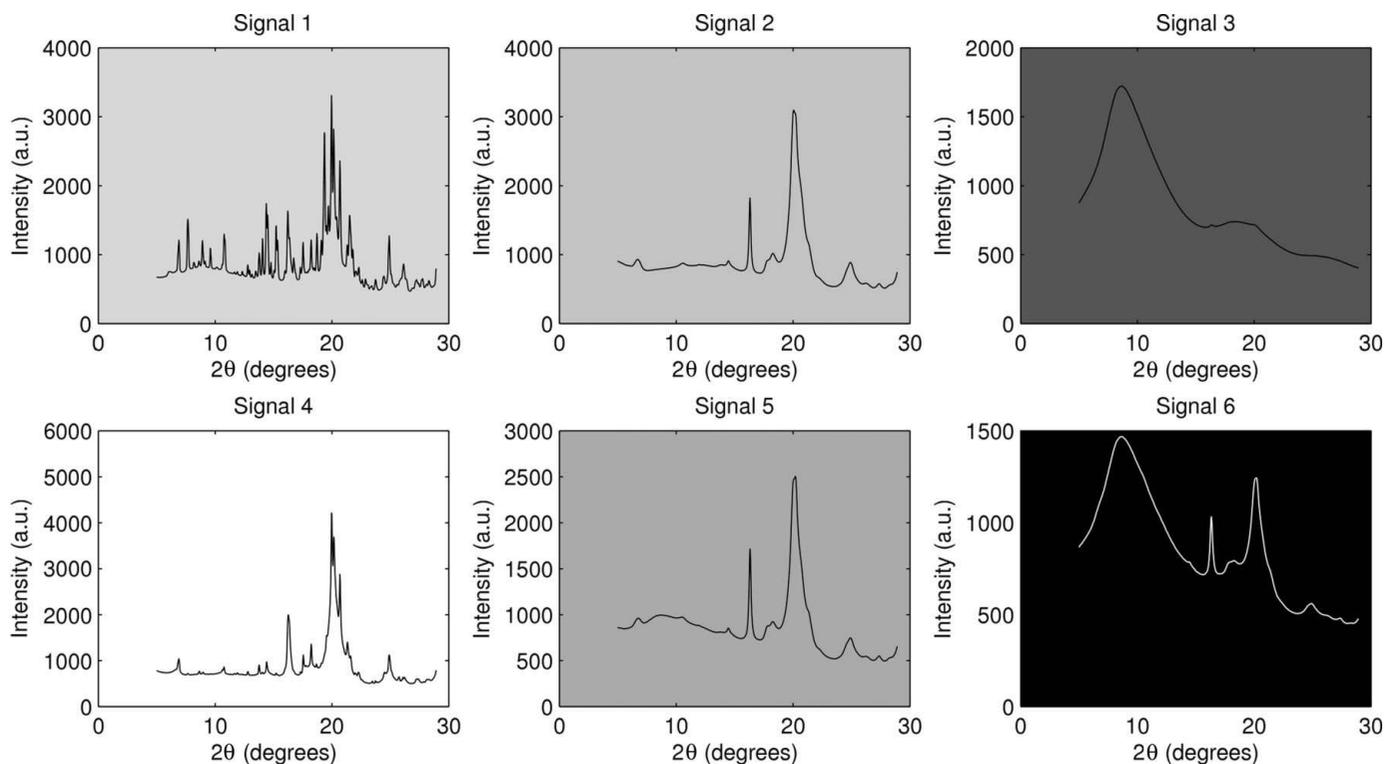
**Figure 2** Characteristic microdiffraction XRD signals of length  $N = 1024$  considered in the simulation studies. They represent a mixture of four crystalline phases (Ha-nano, Ha-micro, Si-Tcp,  $\beta$ -Tcp) and the sample bulk (amorphous) according to the weight percentages as reported in Table 1.
